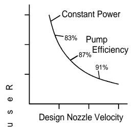
The resulting thrust force from a given amount of hydraulic power is the best measure of propulsion efficiency. It is clear from this that the highest thrust force results from the design based on the lowest pump efficiency due to the much higher fluid power transfer efficiency.
