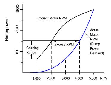
You can see that the motor must run at nearly twice its most efficient RPM to deliver power to the efficient pump. This results in 20% to 30% more fuel consumption. The more efficient total system again uses a less efficient pump that can provide continuously variable power transmission to operate the motor more efficiently. The following graphic shows the more efficient motor power demand curve resulting from this compromise.
